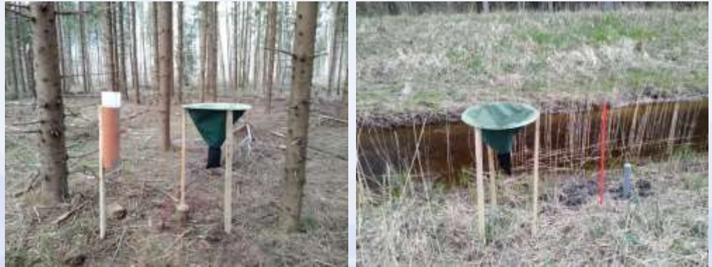
Planned measures (above), example of monitoring points along Åge tributary Tora (left) and monitoring equipment – precipitation, litter and groundwater samplers
