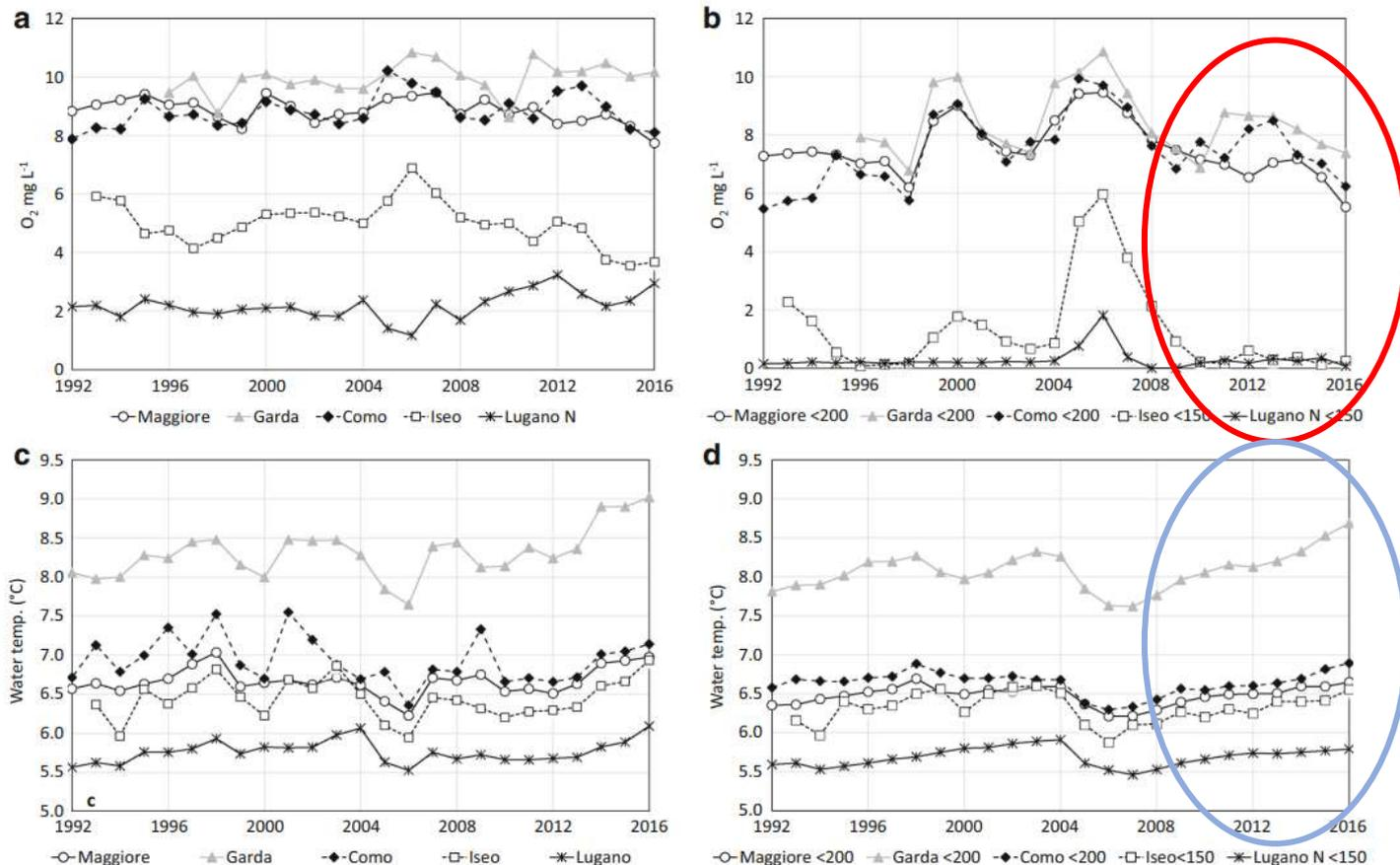
**Fig. 2** Trends of oxygen concentrations and water temperature in the DSL in the period 1992–2016. Average values of DO and temperature in the water column (a, c) and in the deep layer (b, d) measured during winter–spring turnover (usually in March)
