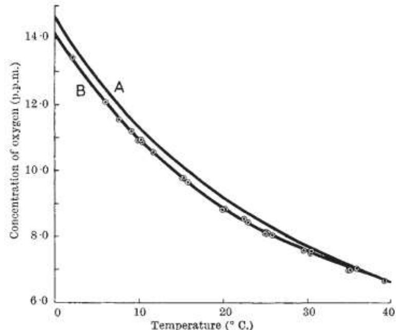
Fig. 1. Curve A, saturation values taken from "Standard Methods" calculated by Whipple and Whipple on measurements made by C. J. J. Fox (atmosphere assumed to contain 20.9 per cent oxygen); curve B, saturation values determined by the Winkler method
